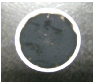
Figure 14 - Effective facial area of sample filter (file photo, not from the evaluation in this report)
