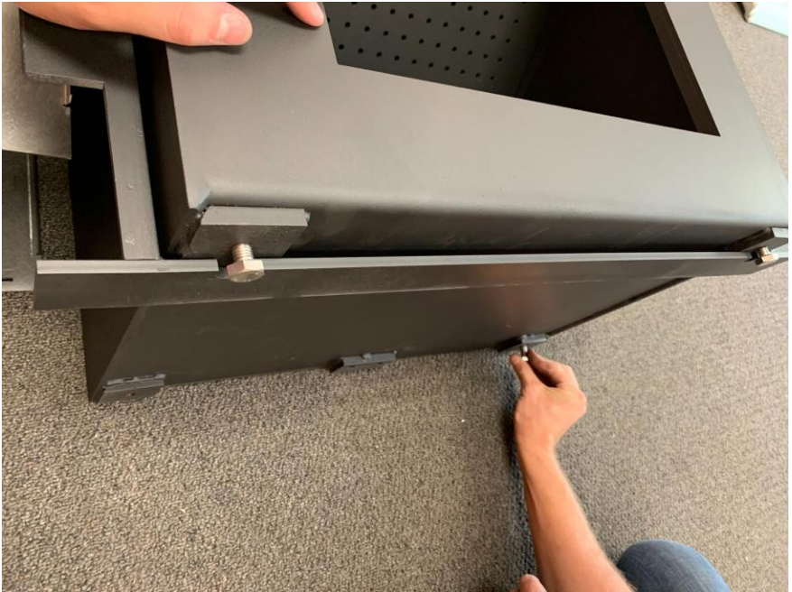
Attach Leg Pad Bolts to bolt holes on the legs of the stove.
