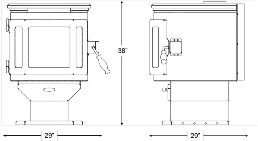
All clearances, side, corner, and back, are measured from the largest dimensions.
