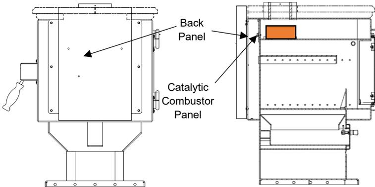
To access the catalytic combustor, first remove the back panel of the stove, then remove the catalytic combustor panel. The catalytic combustor (orange) may then be lifted up and removed from its ring holder. If any cracking or peeling is observed, the catalytic combustor must be immediately replaced. Please contact MF Fire for a replacement catalytic combustor.
