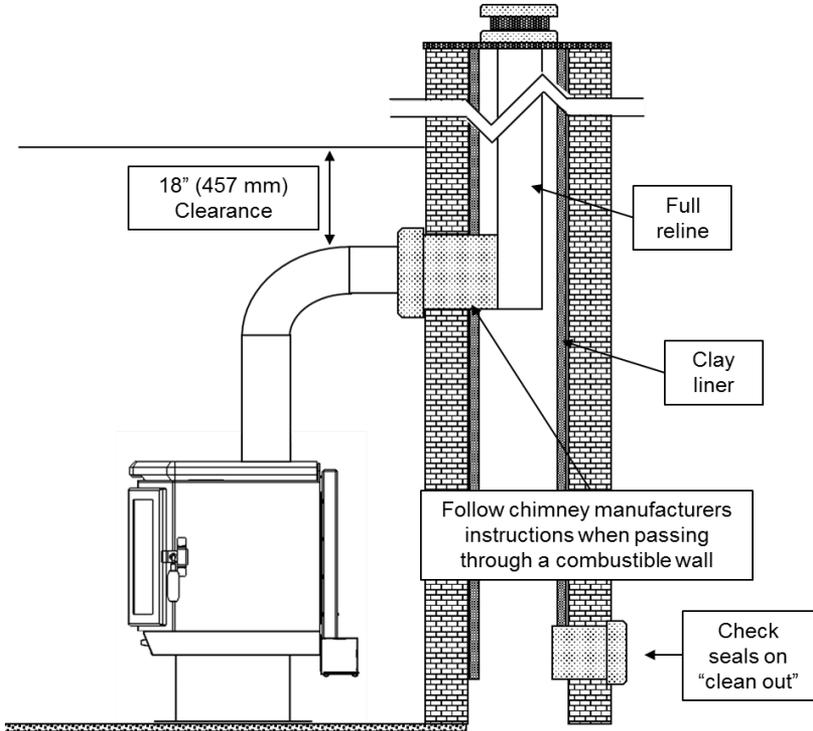
Special care must be taken regarding the wall thimble, or penetration from the chimney connector pipe to the masonry chimney, if the wall thimble must pass through an exterior wall. Here all chimney manufacturer's instructions must be followed, including guidance on spacing to combustible surfaces, piping requirements, and liner requirements. Check with local authorities before installation to ensure all requirements are met.
